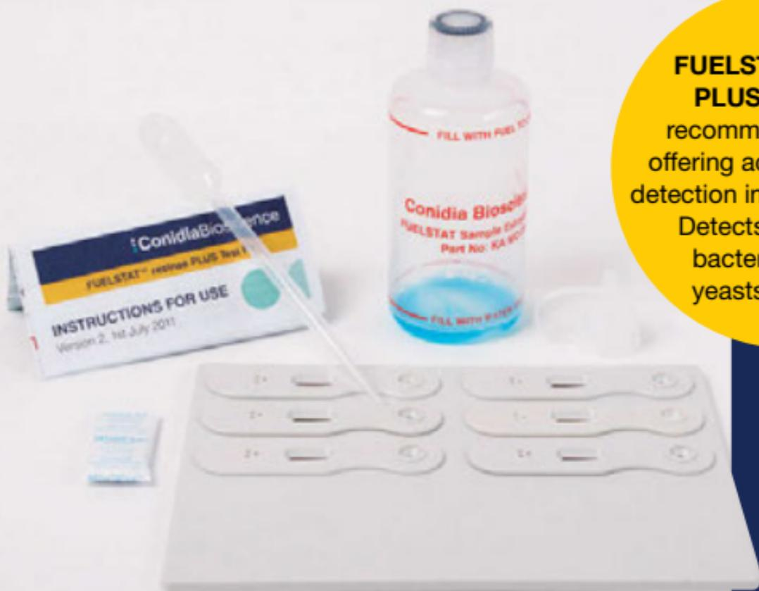
**FUELSTAT® resinae PLUS** – The IATA recommended test kit offering accurate, on-site detection in just 10 minutes. Detects and reports bacteria, moulds, yeasts and H.res.
